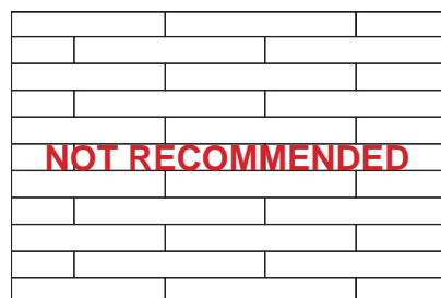
Brick bond installation 50% (NOT RECOMMENDABLE)
