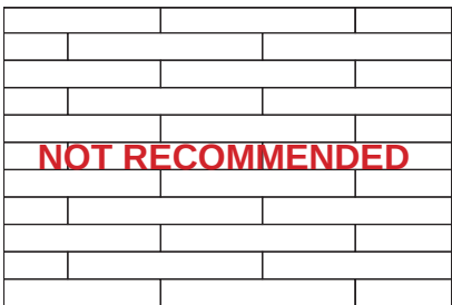
Brick bond installation 50% (NOT RECOMMENDABLE)
